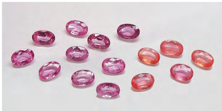
Figure 3. The Be-diffusion process is capable of causing dramatic changes in the color of corundum, such as altering pink sapphire (left, before treatment) to pink-orange (right, after treatment). The samples weigh approximately 1 ct each; photo by Sriurai Scarratt.
