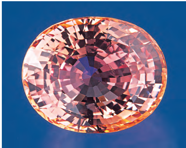
Figure 33. Not all sapphires treated with beryllium have an intense color, as this 14.38 ct Be-diffused sapphire illustrates. It has a medium tone very similar to that of some natural-color sapphires. It is interesting to note that the thin orange layer present in this stone is visible even without immersion, which is not usually the case. Photo by Maha Tannous.
