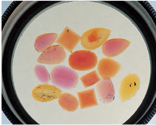
Figure 35. A wide variation in the penetration depths of surface-conformal color layers can be seen in this group of faceted Be-diffused sapphires (0.51–1.92 ct), immersed in methylene iodide. Photo by Maha Tannous.
