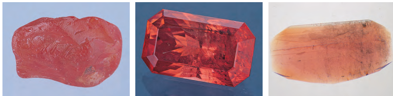
Figure 39. A Be-diffused stone will not always have a complete surface-conformal layer of color, which could cause confusion with natural color zoning. We had the diffused piece of rough on the left cut into the 1.74 ct stone in the center. As can be seen with immersion on the right, the orange diffusion layer was evident only as concentrations just under the surface along the edges of the table and one side of the pavilion, and not all the way around the stone. Left and center photos by Maha Tannous; photomicrograph on the right by Shane F. McClure, magnified 10 \times .
