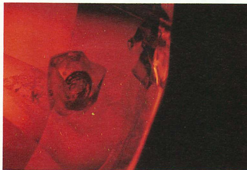
Thai ruby: magnified view (46 times left and 60 times right) of a surface pit which has been repaired by filling it with a glassy material. Note the large gas bubble in the filling material. The discovery was made by Suree Charoensrihanakul.
